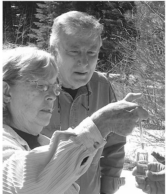
Donna Shorts and Ron Szymanski titrate a sample to measure dissolved oxygen.
